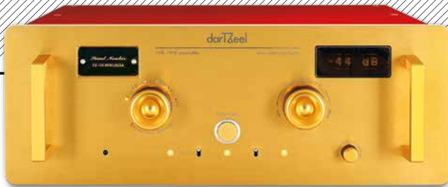
ABOVE: NHB-18NS's substantial rotaries govern input selection ('Enjoyment Source') and volume ('Pleasure Control', calibrated in \pm 0.5\text{dB} steps) while three LEDs indicate stereo/mono operation, battery charging status and mute. Other idiosyncratic messages appear on the yellow display...
