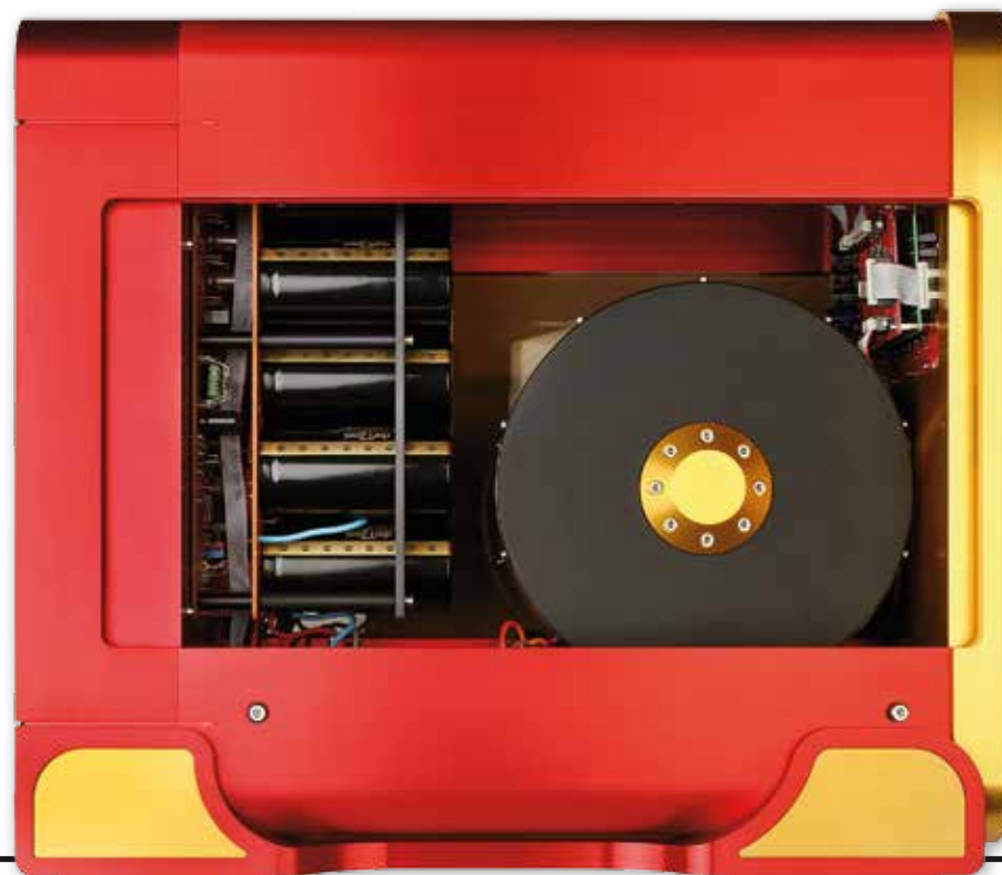
BELOW: Massive 2kVA transformer and 10x 15,000 \mu\text{F} /160V reservoir caps support the NHB-468 power amp – all mounted on a 'floating' subchassis [transit bolts shown here]
