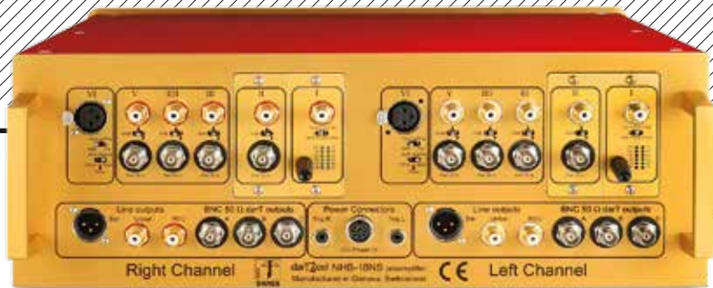
ABOVE: Balanced XLR and four single-ended inputs (on RCAs and 50ohm 'Zeel' BNCs) offer three gain settings while loading/gain configuration for the MC phono input is achieved by multiple clicks of a toggle switch. A full six pre outs are offered on XLR, RCA and 50ohm BNC connections while battery DC PSU is connected via a DIN lead
