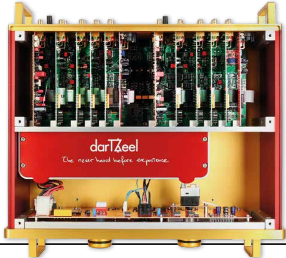
RIGHT: Line and MC phono stages – all 6-layer PCB 'cards' with onboard logic – are mounted onto a backplane for ease of servicing/upgrade. Volume is also logic-controlled but CPUs 'sleep' if the IR handset, knobs or toggles are not in use
